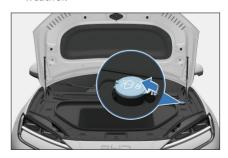
When refilling the washer fluid, use a clean cloth dipped in the windshield washer fluid to clean the windshield wiper blade. This helps keep the wiper blade in good condition.
