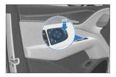
To enable or disable side mirror auto fold and auto tilt while reversing functions, go to infotainment touchscreen  $\rightarrow \boxminus \rightarrow Vehicle \rightarrow$ Comfortable Use
