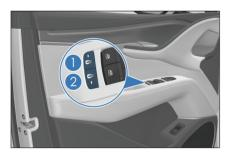
After the child protection lock is activated, doors cannot be opened from inside the vehicle, and the window switch for the corresponding rear door cannot be used to raise or lower the window. To unlock the door, press the child protection lock button for the corresponding side again or use the exterior door handle.
