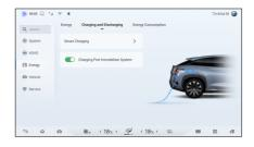
· When the immobilizer is activated, the charging connector will lock if charging connector is connected and the four doors, hood and trunk lid are locked. To disconnect the connector, unlock the vehicle first
