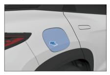
Open the charge port cap (configurations of the actual vehicle prevail), and make sure that no obstacles exist between the head of the charging connector and the end of the charging socket.
