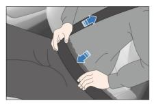
3. Insert the latch into the buckle until it clicks, and then pull it back to make sure it is firmly locked. Do not fasten the belt with any part of the strap twisted.
