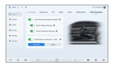
When the system sounds a fatigue or distraction warning, pressing the scroll button on the steering wheel pauses the warning for 15 minutes, during which no warnings will be given.
