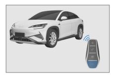
3. Press and hold the remote start/stop button on the electronic smart key for two seconds. The vehicle powers off, and turn signals flash twice.
