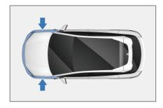
The airbag cover (highlighted area shown) has been scratched, cracked or otherwise damaged.
