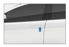
• If any door, hood, or trunk lid is not closed, pressing the microswitch still locks the closed doors, but the alarm only sounds once, and the side mirror do not flash.
