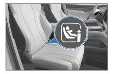
The front passenger seat is equipped with a top tether anchorage on the back.
