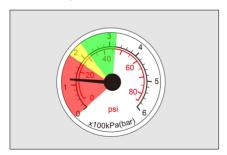
If the tire pressure reaches between 180 and 320 kPa (green and yellow areas shown in the illustration), remove the kit as soon as possible and drive at a speed below 80 km/h within one minute, with the furthest driving distance not exceeding 10 km, so that the tire sealant is evenly distributed within the tire.
