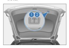
Press this button a second time to stop the lid at the current position. Press this button again to have the lid move in the opposite direction.
