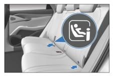
The outboard rear seats are equipped with top tether anchorages on the back.
